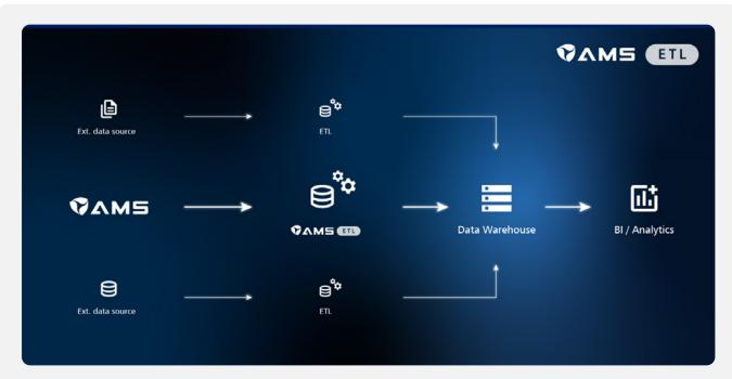
Data from AMS as well as from other systems is extracted, transformed into a suitable data structure, and loaded into the Data Warehouse (DWH). It stores all data in a universally readable Snowflake schema\*, which allows access for external Business Intelligence applications such as Power BI. This enables comprehensive evaluations that can be summarized in clear reporting dashboards.
